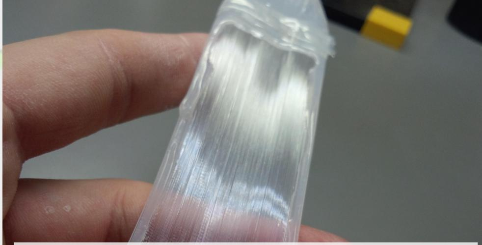
The trigger must have a lower density for Cherenkov radiation condition. By using the fiber of 0.2 mm in diameter, the energy loss can be reduced.
