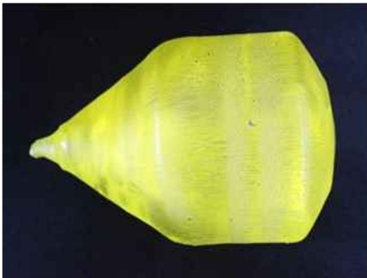
Fig.1: Photograph of 3-inch-diameter GAGG scintillator.
