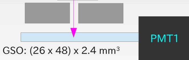
$$\text{Resolution } dE = \frac{\sigma}{\mu} \sim 0.1$$
