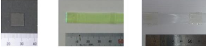
Fig. 3. The La-GPS crystal (left) with the thickness of 0.50 mm is used as a scintillator. The Y-11 (300) MJ WLSFs (center) and the B-3 (300) MJ WLSFs (right) are 0.2 mm in diameter. They are arranged in sheet-like.
