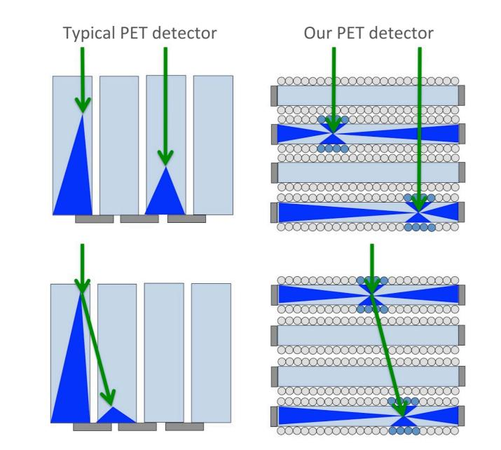
In this study, the detector performance for 511-keV gamma ray is demonstrated by an experiment.
