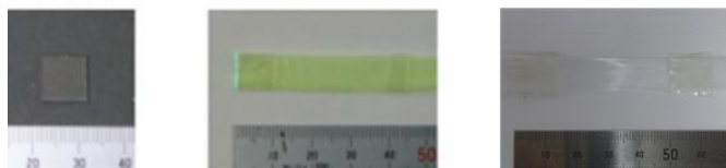
Fig. 3. The La-GPS crystal (left) used as a scintillator. The Y-11 (300) MJ WLSF (center) and the B-3 (300) MJ WLSF (right) are 0.2 mm in diameter. They are arranged in sheet-like.
