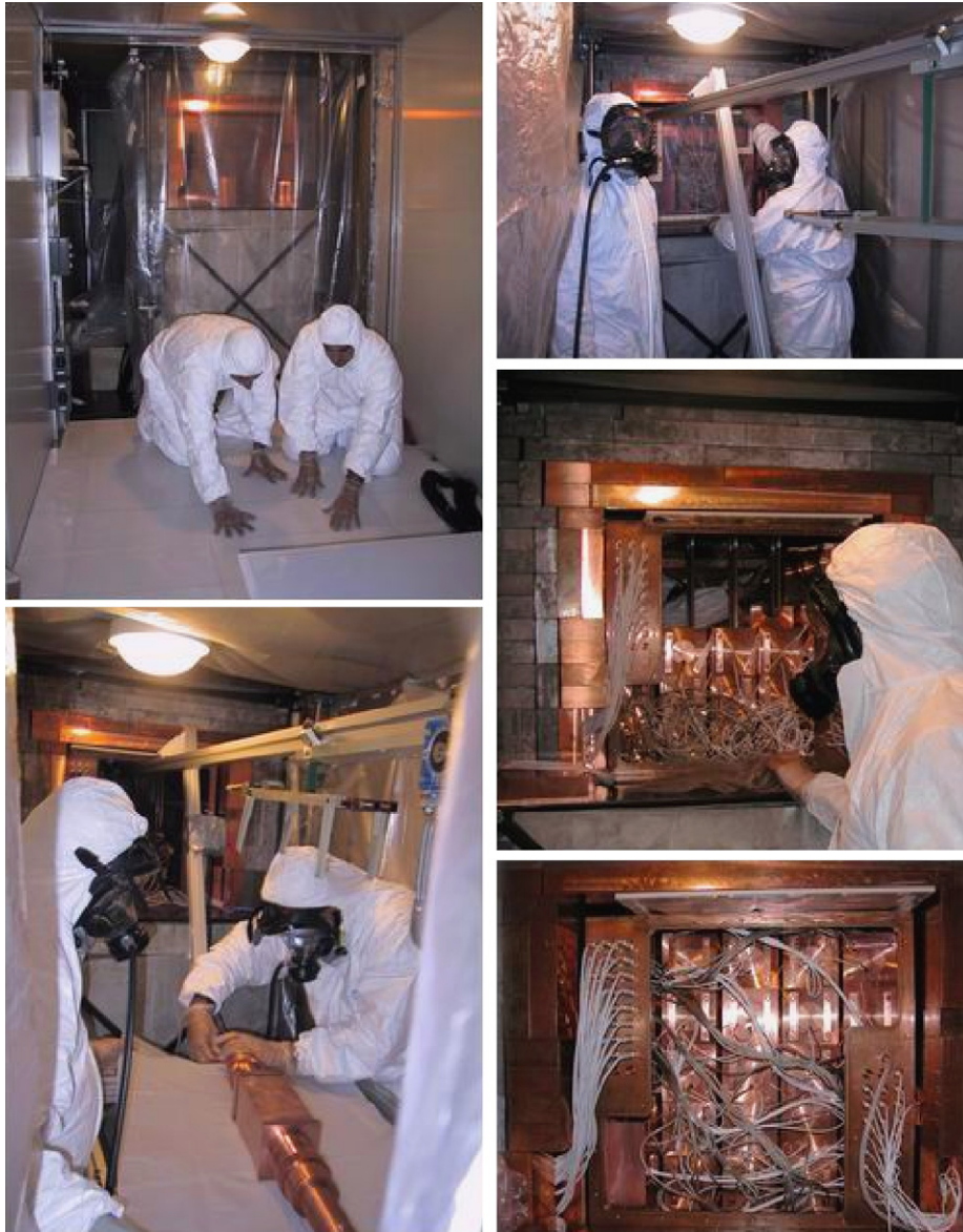
Fig. 1. Disinstalling DAMA/NaI and installing DAMA/LIBRA; all procedures involving detectors, photomultipliers (PMTs), etc. have been carried out in HP (High Purity) Nitrogen atmosphere. Improving the experimental site (walls, floor, etc.) after removal of the DAMA/NaI electronics ( top left ); dismantling the DAMA/NaI detectors in HP Nitrogen atmosphere ( top right ); assembling a DAMA/LIBRA detector in HP Nitrogen atmosphere ( bottom left ); installing the DAMA/LIBRA detectors in HP Nitrogen atmosphere ( center right ) and a view of the inner Cu box filled by the DAMA/LIBRA detectors in HP Nitrogen atmosphere ( bottom right ).
