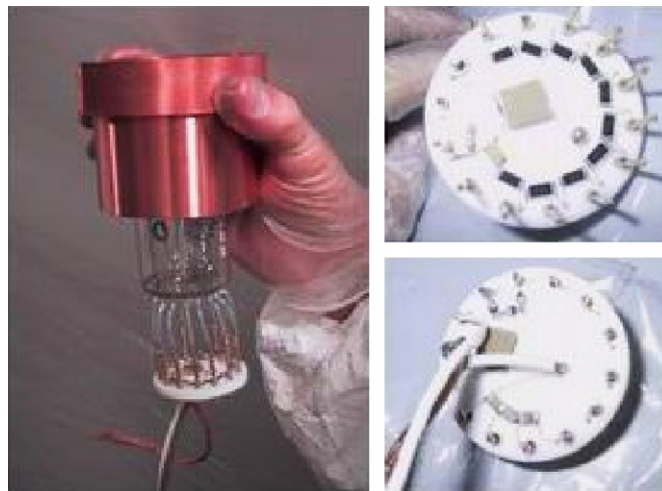
Fig. 12. Left: A DAMA/LIBRA PMT with flying leads directly connected to the voltage divider. Right: A voltage divider assembled with miniaturized SMD resistors and capacitors mounted in thin teflon socket.
