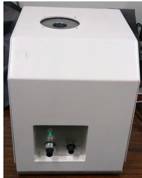
Fig. 4. Developed GAGG well counter system. Sample is set inside hole of upper side of counter. High voltage supply is included in system.
