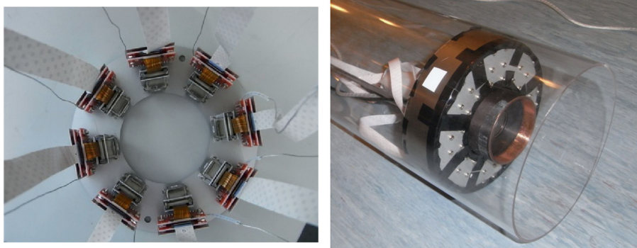
Fig. 8. The prototype gantry for MRI-PET. This gantry consists of eight MPPC-based PET modules, and is made of titanium and aluminum.
