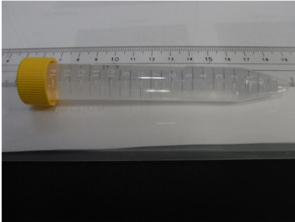
Fig. 4. The phantom used for MR imaging tests. This plastic cylinder filled with water.
