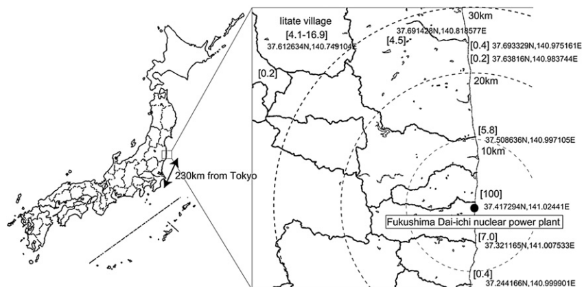
Fig. 4. Sampling sites and spatial dose of radiation. The value in square brackets, such as [100], is the value of the spatial dose of radiation ( \mu\text{Sv h}^{-1} ) 1 m above ground on the day of sampling (April 10, 2011).
