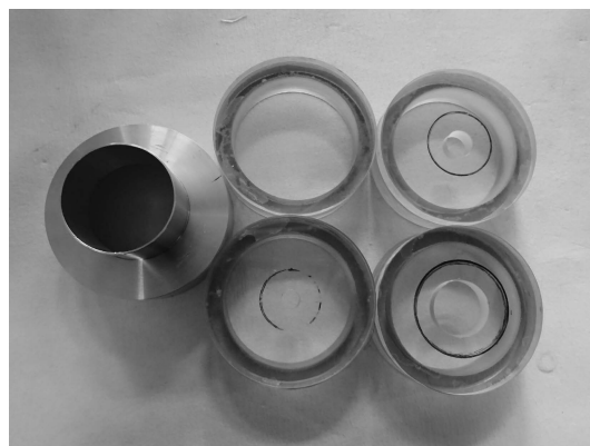
Fig. 3 Picture of acrylic resin collimators and aluminum holder used for measurement
