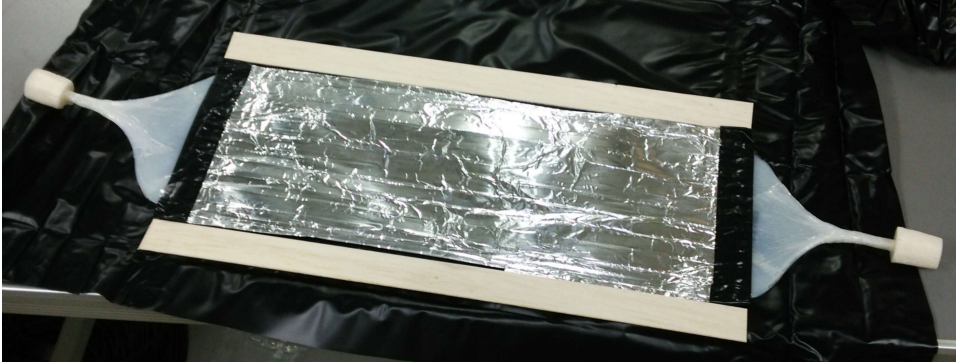
Fig. 3.4: The \beta -ray counter based on scintillating fibers with an effective area of 30 \times 10 cm.
