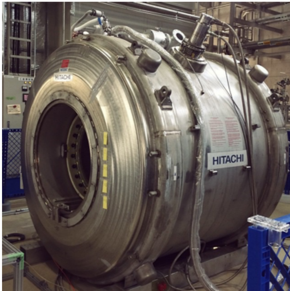
Superconducting magnet at J-PARC, Tokai
