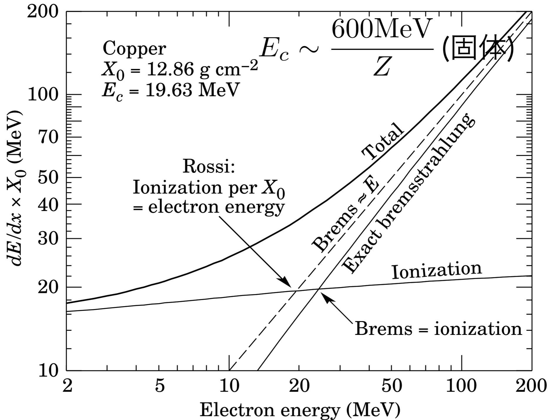
**Figure 33.13:** Two definitions of the critical energy  $E_c$ .
