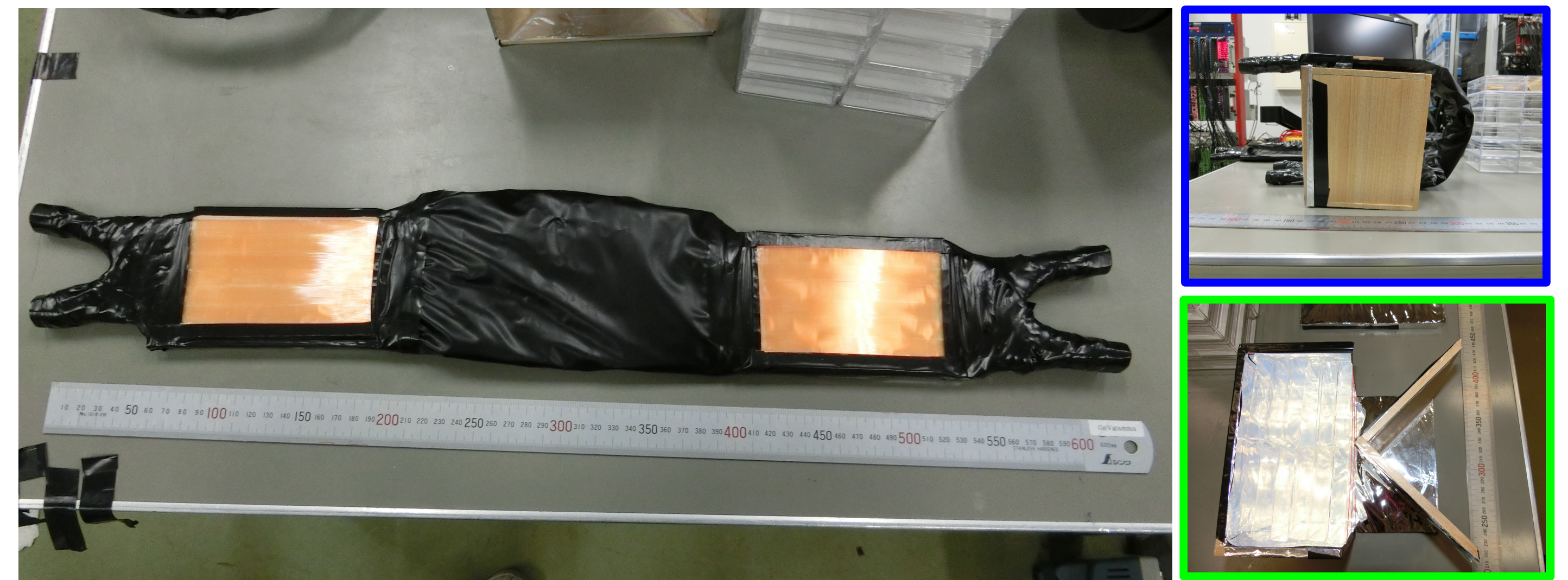
Fig. 2: The light guide has two sensitive faces with the fibers (left) and two side faces are covered with it (top right). A box has a V-shaped reflector and internal. Total aerogel size is (120 mm x 90 mm) x 60 mm (bottom right).
