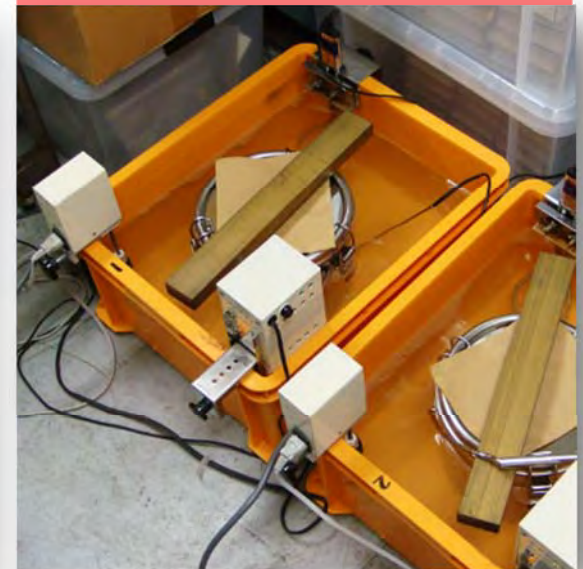
2nd aging using a water bath at 35°C
